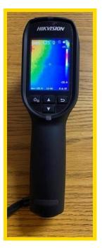
This handheld thermal scanner is portable, measures temperatures, and records images directly to a micro SD card - eliminating the manual recording of information. This user-friendly and cost-effective scanner can be implemented at short notice.
